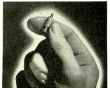
Fig. 3—Typical crystal for converter stage.
