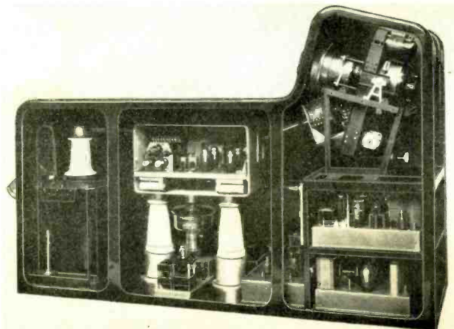
Fig. 4—Side view of the projector with cover removed to show arrangement of the components.
