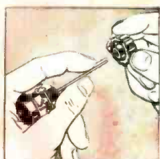
Use half the U-clip to hold push-on type knobs.
