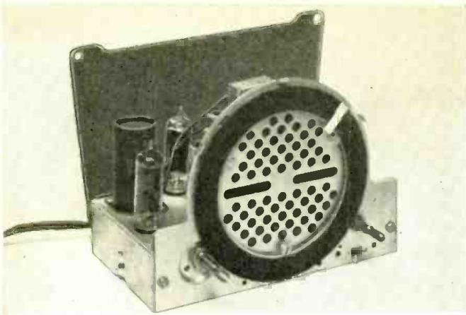
Fig. 1—The dial pointer is on the ring in front of the speaker.
