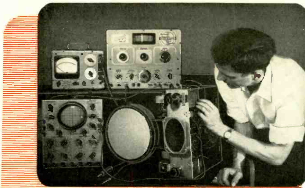
Instruments set up properly to align a television receiver.
