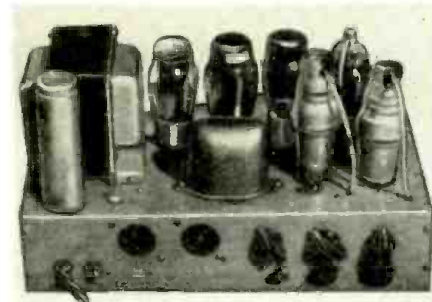
Fig. 3 (above)—The 6-tube, 13-watt amplifier. Fig. 4 (left)—Chassis layout of this unit.
